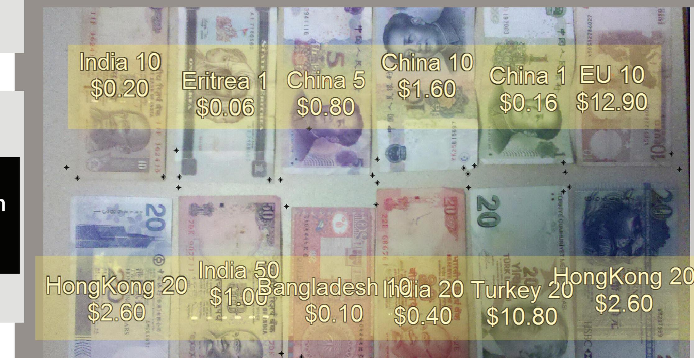
14 bills (front & back) can be detected, distinguished and totalled. Up to 12 bills can be detected at once. Overlapping and similar bills can be properly detected.
