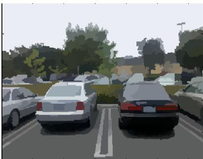
**Figure 5: An example of excellent plate separation by mean-shift segmentation. Note that without prior knowledge of candidate region size, the segmentation would not produce such a desirable result in many cases.**
