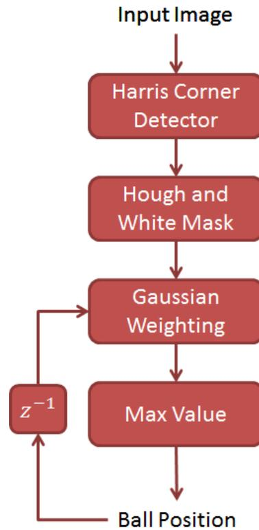
Figure 7: Flowchart of Ball Detector
