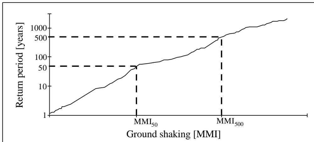
Figure 4.2. Schematic example of a hazard curve
