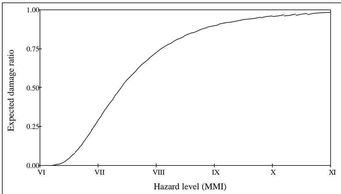
Figure 3.2. Schematic example of a damage curve. Based on RMS (1997).
