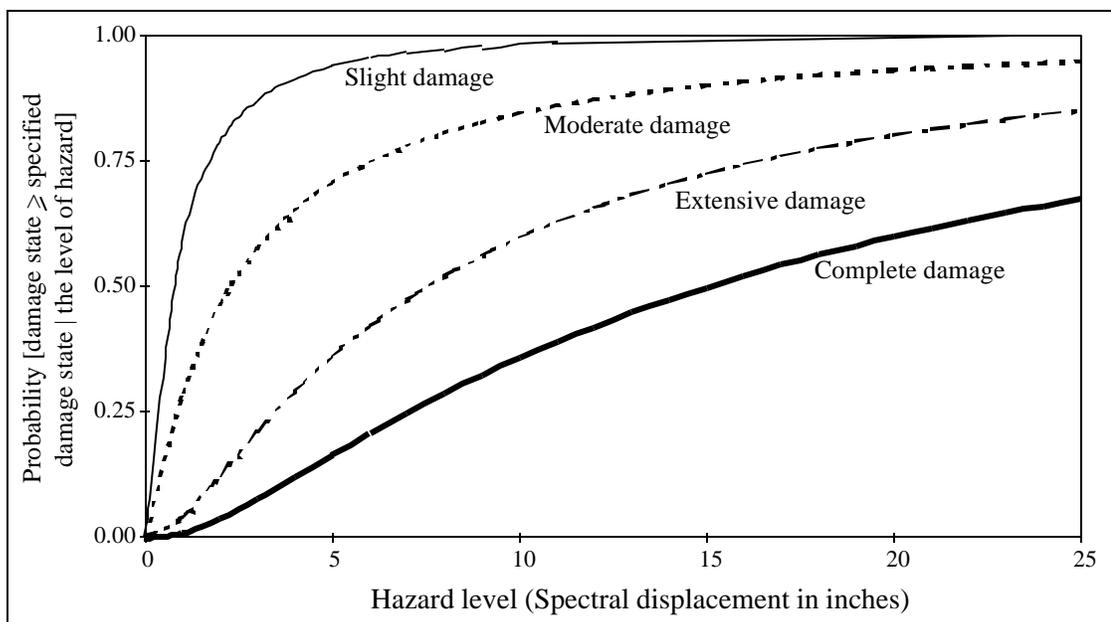
Figure 3.3. Schematic example of a set of fragility curves. Based on RMS (1997).
