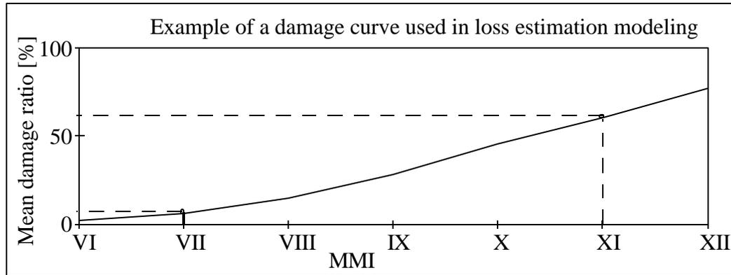
Figure 4.4. Example of a loss estimation model damage curve
